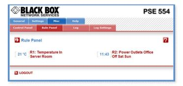
For supervision purpose, the administrator can create special accounts which display only some specific rules. In the example below, the user Bill has the possibility to supervise 2 rules and to see on a glance the rules which have been triggered.
