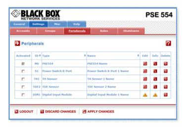
The Peripherals page is used to configure all peripherals connected to the Power Switch 4-port.
