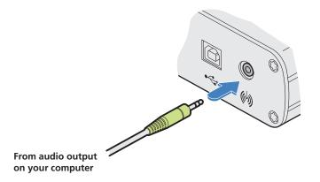
Figure 3-3. Connecting an audio cable to the local module.
