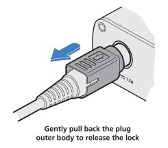
Figure 3-16. Disconnecting the power adapter plug.
