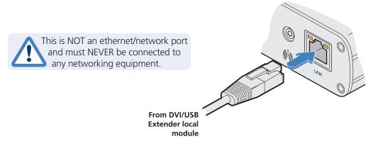
Figure 3-13. Connecting the remote data link on the rear panel.
