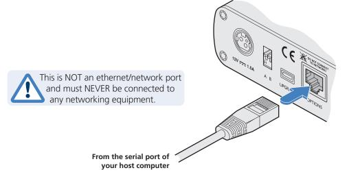
Figure 3-4. Connecting a serial cable to the OPTIONS port on the local module.
