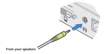
Figure 3-11. Connecting speakers on the rear panel.
