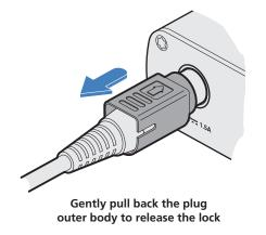
Figure 3-7. Disconnecting the power adapter plug.
