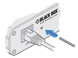
Figure 4-2. Press and hold the recessed reset button for approx 10 seconds.
