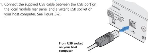
Figure 3-2. Connecting a USB link to the local module.
