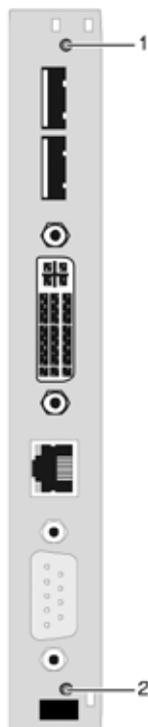
FIGURE 2-7. STATUS LEDS ON CPU BOARD (ACX288-R2-CTL)
