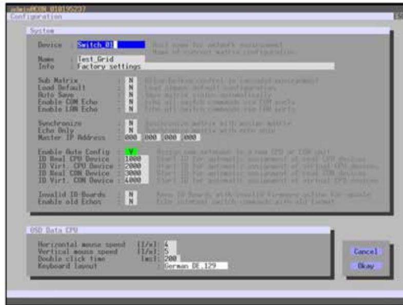
FIGURE 4-65. CONFIGURATION—SYSTEM
