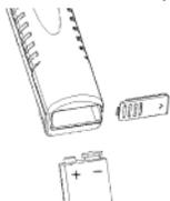
Remove the battery cover at the bottom of the unit and insert the battery with the terminal orientation as shown. Battery polarity is marked on the back of the battery cover and inside the battery well for reference.
